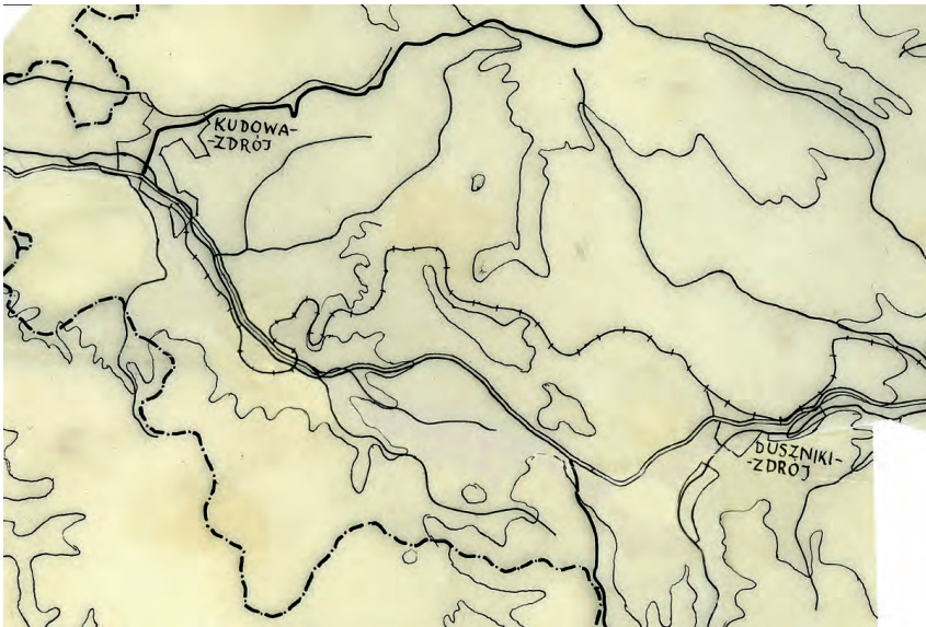
Fig. 5a. The first stage of preparing the manuscript of The Kłodzko Land map. The figure shows a fragment of the drawing of basic elements of the map content, which was made in the scale of 1:75 000 (original scale) based on cartometric sources
