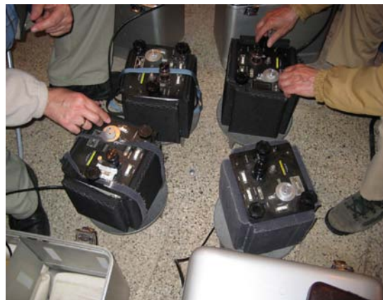
Rys. 6. LaCoste&Romberg gravimeters inside styrofoam shields
