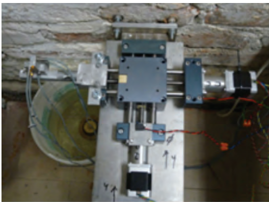
Fig. 5. The inductive device without its housing at a test stand
