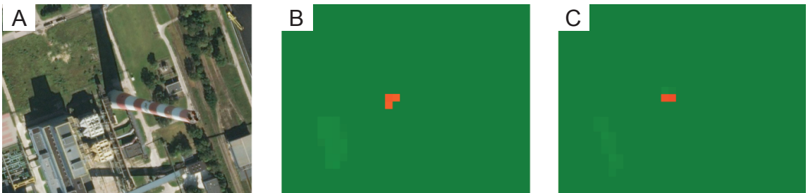
Fig. 5. The example of the outlier – the height of the chimney: B – based on BH2012 (three pixels) and C – based on the LIDAR data (two pixels) with the orthophoto basemap (A)
