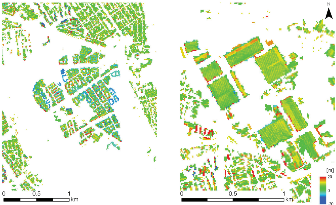
Fig. 2. Subtraction of the Building Height 2012 layer from the LIDAR data
