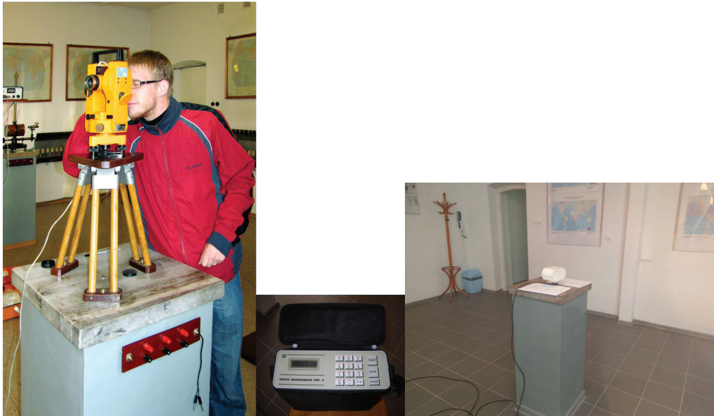
Fig. 5. The measurement of magnetic declination, inclination and module F of the total intensity vector on the base pillar in Belsk observatory
