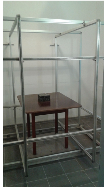
Fig. 3. The coil developed in the Central Geophysical Observatory of the Institute of Geophysics of the Polish Academy of Sciences in Belsk used to check the proton magnetometer
