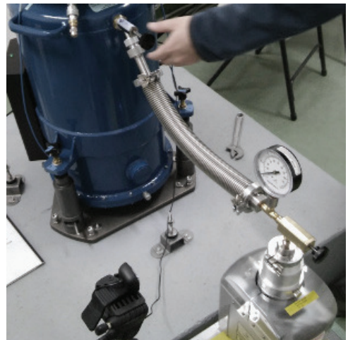
Fig. 7. Pumping the dewar vacuum insulation
