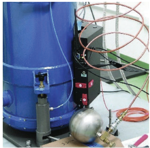
Fig. 5. Approach to solve the issue of Taconis oscillations
